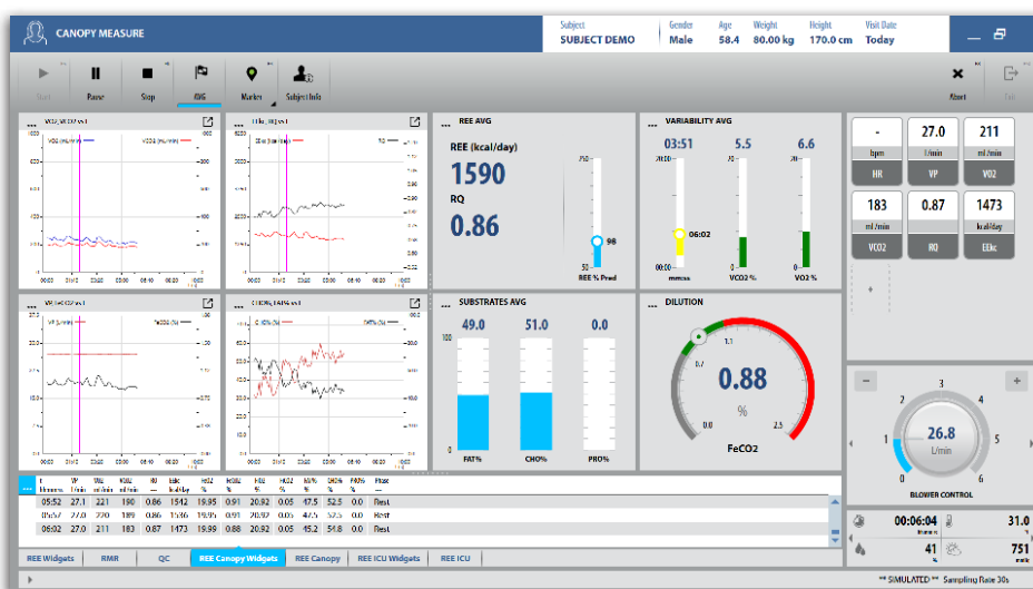
Real time data in Canopy Mode using the optional OMNIA Software. Intuitive gauges help users with quality control and results interpretation.
